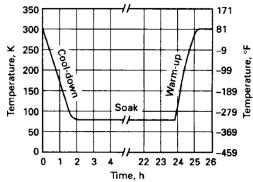
Fig. 1 Plot of temperature versus time for the cryoprocessing process. Soaking temperature is -196°C [7]
